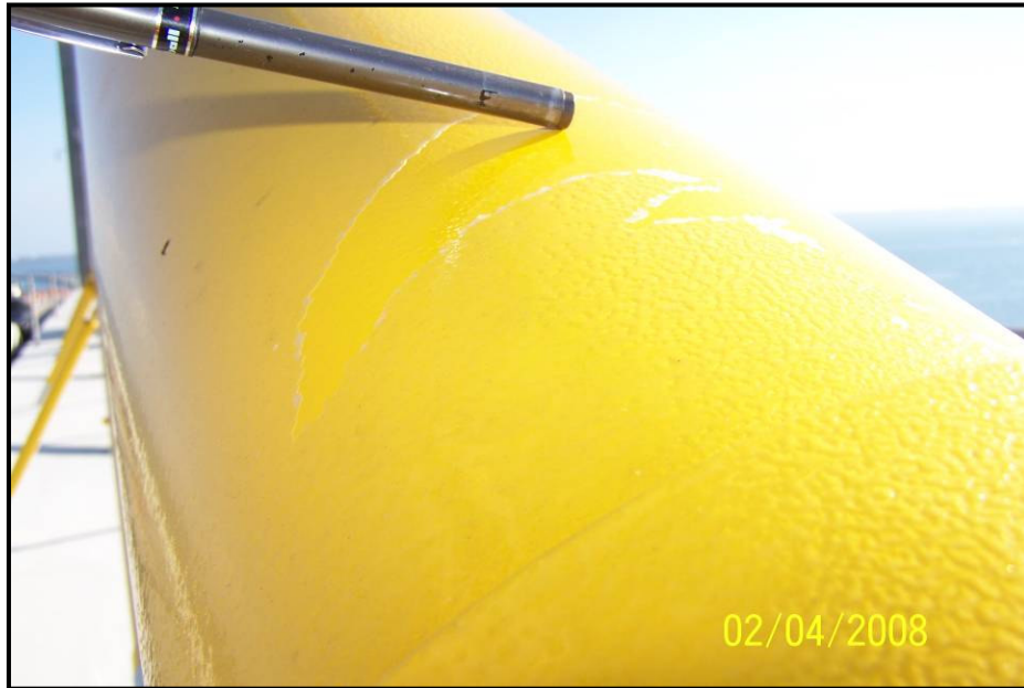
Figure 10- Note the clear pulling away and the thickness and cloudy appearance of the coating.
