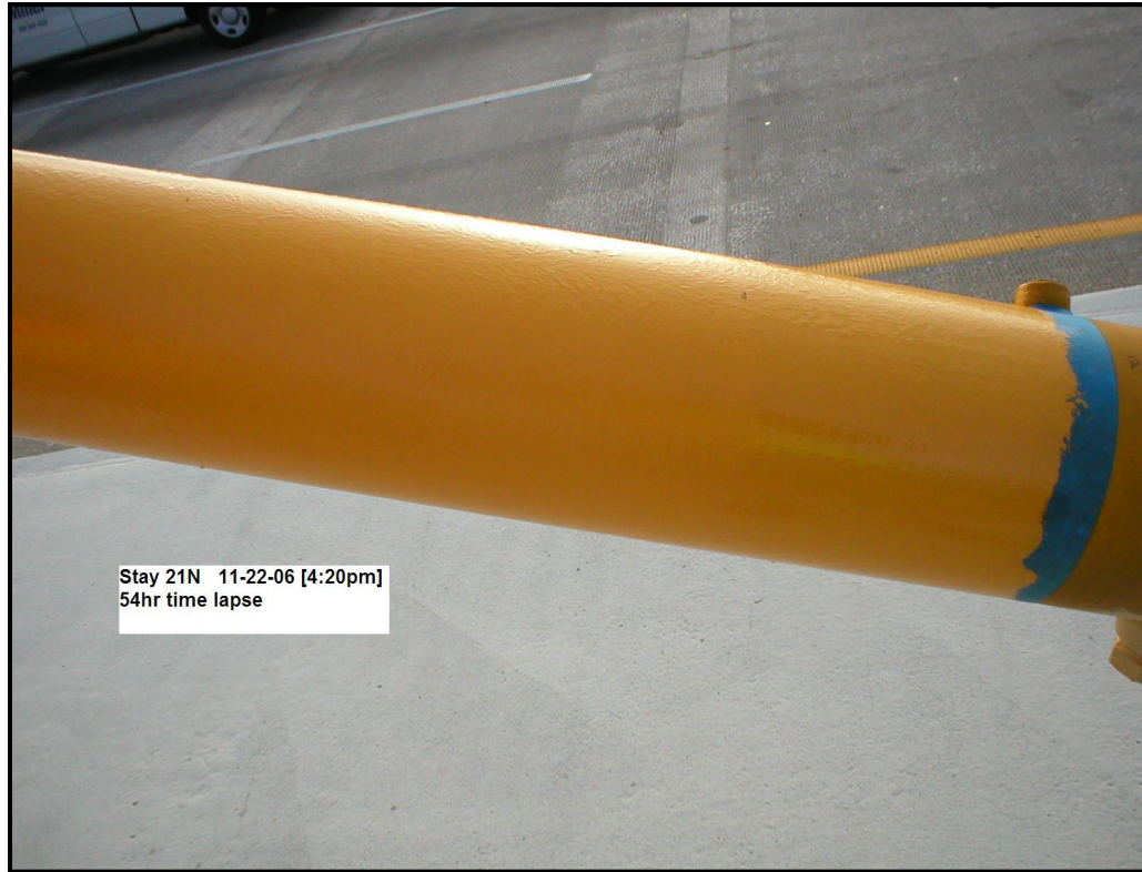
Figure 9 – 54 hour time lapse for dye dissipation.
